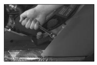
1. Remove the first bolt. Then remove the remaining plastic fasteners holding the shield. Use the end of a flat-head screwdriver to pull up the center of the fastener. Be careful not to break the fasteners that hold the shield in place.
